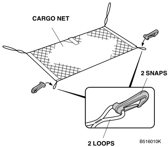
2. Install the cargo net to the anchors and tie-down hooks in the trunk as shown.
