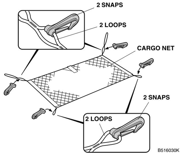
2. Install the cargo net to the tie-down hooks in the trunk as shown.
